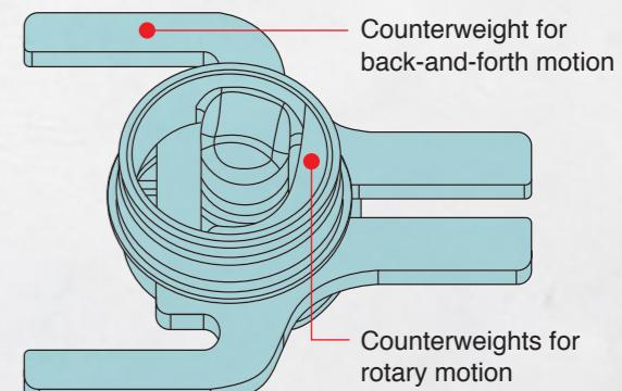
Anti-vibration side grip HR3011FC absorbs excess vibration beyond the canceling capacity of the two counterweights
